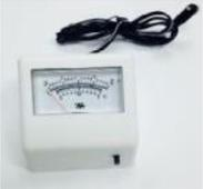
When monitoring with the reverse temperature sensor, the needle moves counter-clockwise with warming.
